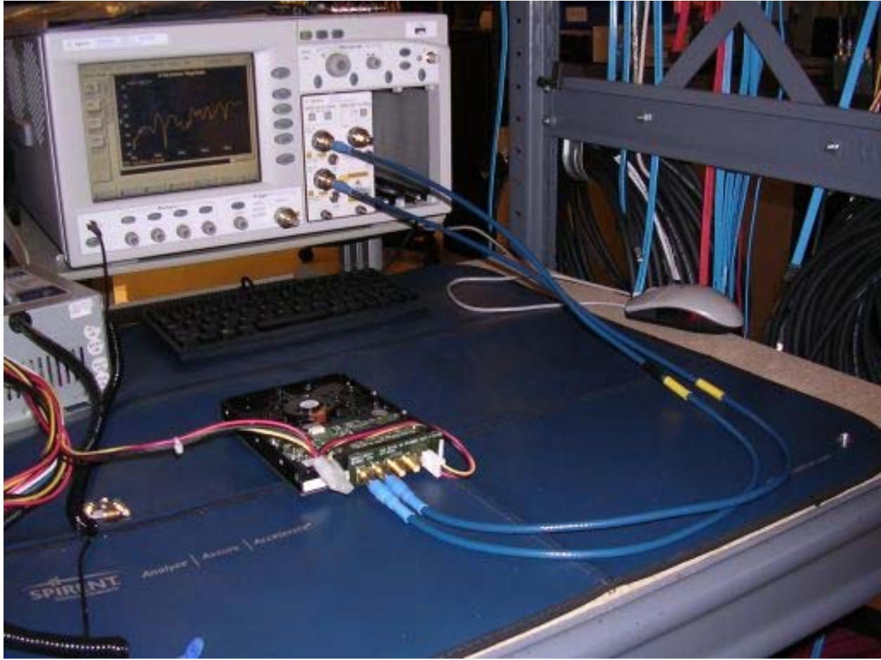
Figure A-3: General TDR Test Setup
