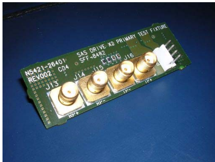
Figure A-1: Agilent SAS/SATA Drive Test Fixture
