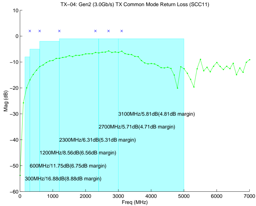
Figure D-10: TX-04 (Common-Mode Return Loss) for Agilent Mated Pair
