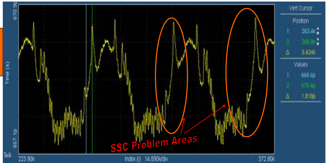
Figure 3 - Violating df/dt (ppm/usec) SSC Profile
