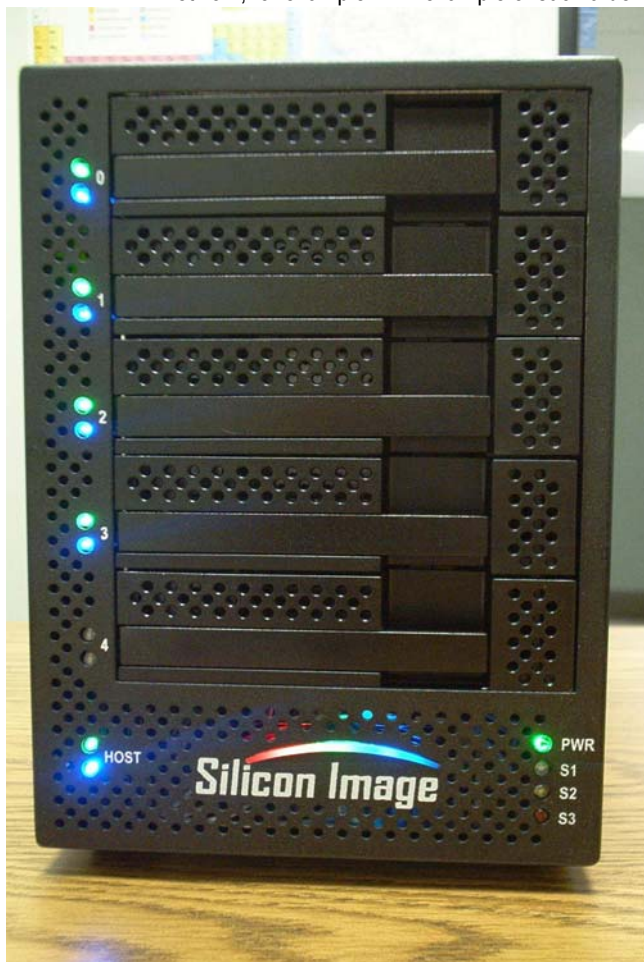
Figure 7: An example of an external storage appliance that uses five standard desktop drives, connected through a port multiplier to a single SATA host connection.
