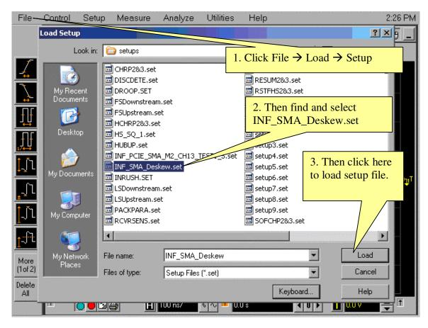
6) If the **INF\_SMA\_Deskew.set** setup file does not exist, it can be recreated from the following setup configuration on the Infiniium oscilloscope.
