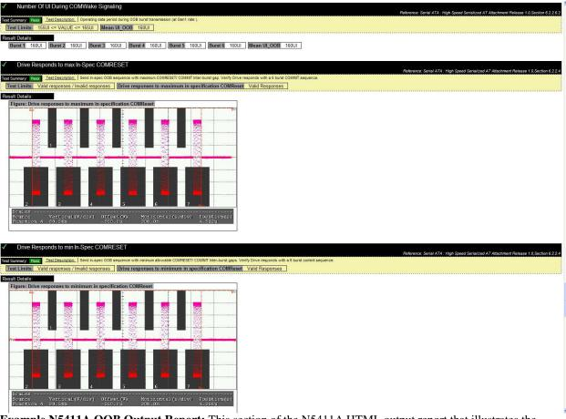
**Example N5411A OOB Output Report:** This section of the N5411A HTML output report that illustrates the pass/fail conditions for OOB-06 and OOB-07 detect/reject tests based on the allowed COMWAKE and COMINIT gap times.
