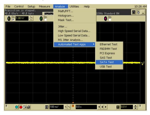
2. Next, choose the type of device that you wish to test (Gen 1i Drive in this example) and associate the 81134A Programmable Pattern Generator LAN connection with the N5411A SATA application.
