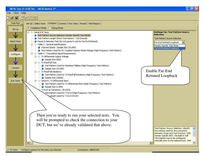
5. Next you will see each one of the tests being performed automatically by the application. A running total of completed tests and a summary of pass/failed tests is also provided. When completed you will see a summary of the test results.
