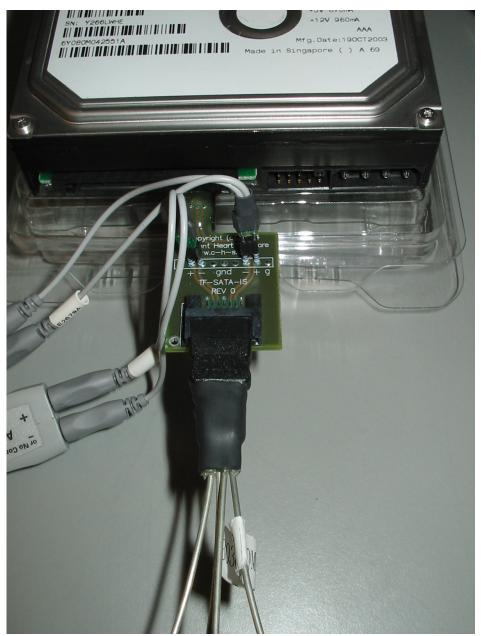
**Example Connection:** Using a Crescent Heart TF-SATA-IS fixture to accommodate probe attachment on the TX/RX lines without disrupting the signaling between the HOST and Device under test.
