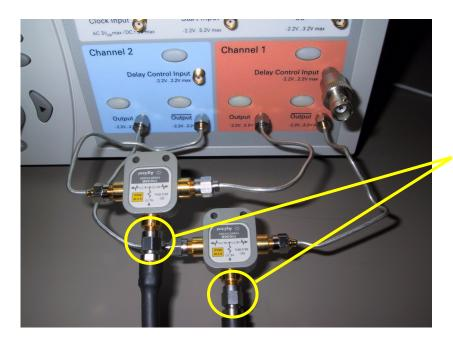
If less than 50mV of differential OOB amplitude is needed at the device receiver, then insert the 33340C 20dB passive attenuators here, one on each of the 11636B power divider outputs, before the SMA cable is attached. The voltage output of the 81134A after the attenuator is now 10 times lower than the voltage selection on the 81134A output. The sensitivity of the adjustment is now 0.1mV instead of 1mV with the divide by 10 attenuator in place.
