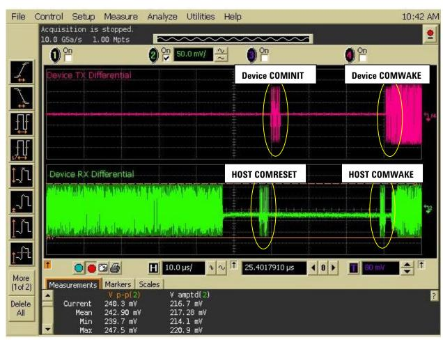
In this figure, the device correctly responds to a valid in-spec COMRESET/COMWAKE OOB initialization sequence at 210mV, thus passing the threshold test. The other requirement for passing is to successfully REJECT the same HOST OOB signal sent at 40mV (for Gen 1i) or 60mV (for Gen 2i).
