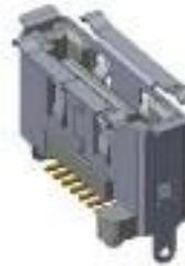
During selection of the right angle surface mount connector, check the pin assignment of the integrated circuit (IC) that the connector will be used with. A reverse configuration is available so that the connector chosen can align with the IC pinout to avoid crossing traces on the printed circuit board layout. The post size and location of the right angle surface mount reverse connector is different than the right angle surface mount connector to prevent installation of the wrong type.
