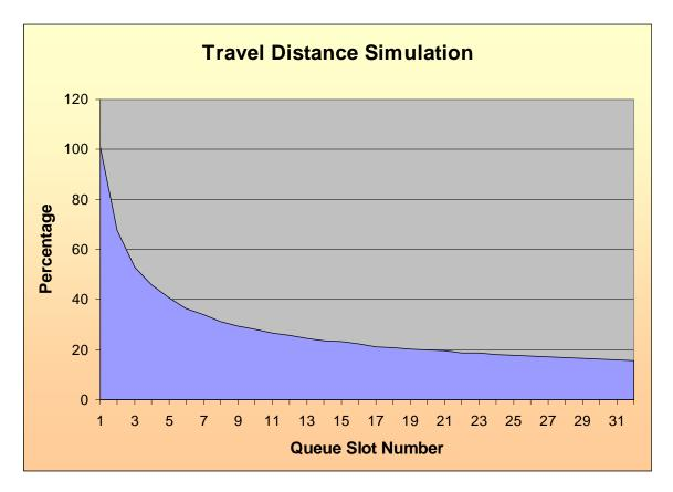
As it shows on the simulated chart, the travel distance is reduced when the slot number increased. When the Queue depth reaches 32, the travel distance becomes 18% of the total distance compare with the 1 slot. This track crossing number reduction can greatly reduce the read/write head movement, and results in a much quieter drive.
