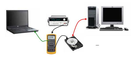
Drive Master 2006 Pro is software from ULINK Technology which is used to send NCQ commands to the hard drive. In this test Drive Master 2006 Pro stimulates the command sequence and the computer connected to the Fluke current meter records RMS current every second. The data of the current consumption is then analyzed and compared.
