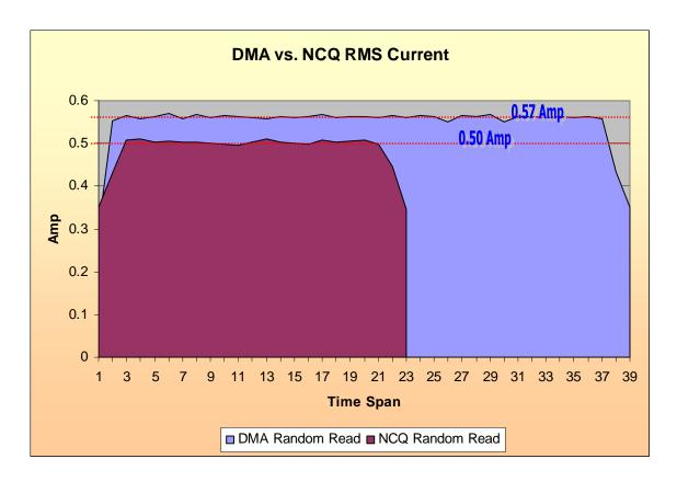
The total power measurement in this test is shown on the chart. A DMA Read consumes 0.57 Amp while the NCQ Read consumes 0.50 Amp. This is a 14% lower current consumption. In addition, by integrating the area, the power wattage DMA and NCQ consumed are 27.264 mW and 18.118 mW, respectively. In other words, NCQ consumes 66.45% of the DMA power usage.
